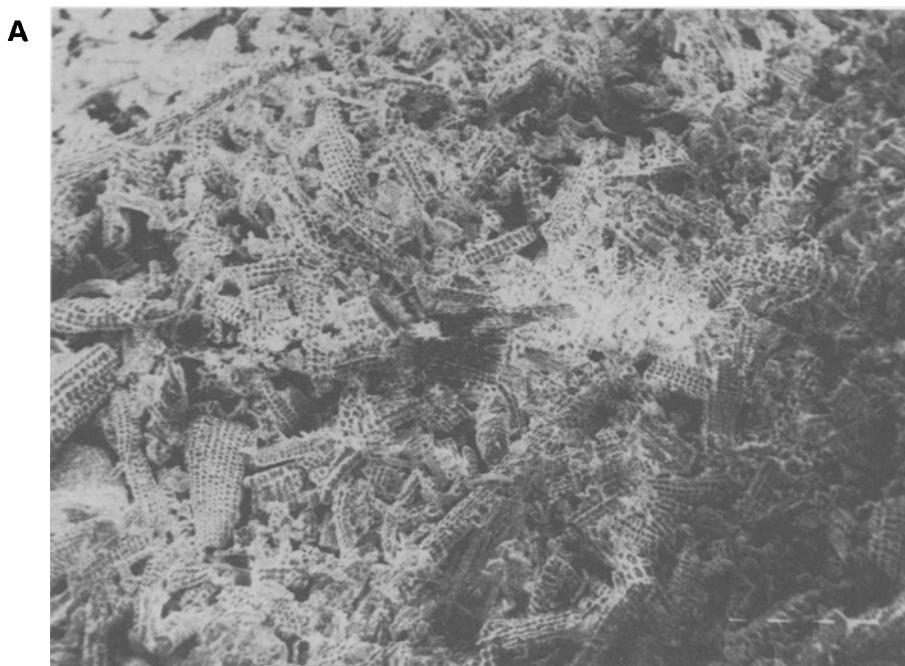
FIG. 7. SEM micrograph of ash heated to 1000°C, magnification (a) \times 20 , and (b) \times 100 (long bar is 100 \mu ).
