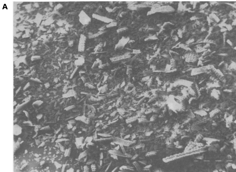
FIG. 5. SEM micrograph of acid activated ash, magnification (a) \times 20 , and (b) \times 100 (long bar is 100 \mu ).
