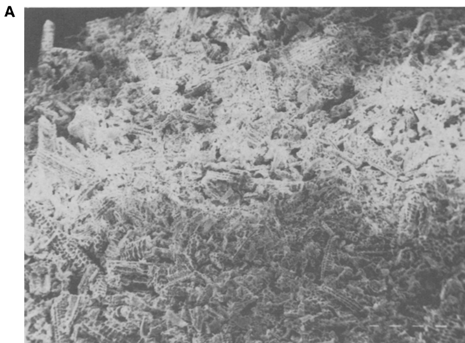
FIG. 6. SEM micrograph of alkaline ash heated to 800°C, magnification (a) \times 20 , and (b) \times 100 (Long bar is 100 \mu ).
